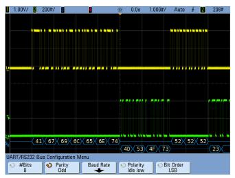
The oscilloscope should now be decoding both the transmit and receive RS-232 signals in hex format. Let's now turn on default RS232 waveform labels so that we can see which analog channel is capturing the transmit data stream and which analog channel is capturing the receive data stream. Let's also set up the oscilloscope to trigger on a specific transmit byte (0x4D). The oscilloscope should currently be triggering on an edge crossing of channel 2 (Auto Scale default triggering).
