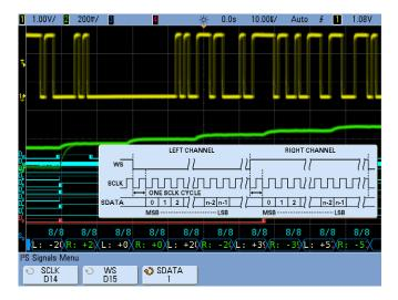
You should now see I<sup>2</sup>S decoding based on 8-bit words of "left" channel and "right" channel data. Note that this might represent stereo information in a digital audio/sound system. Let's now set up the oscilloscope to trigger on a specific transmitted audio data.
