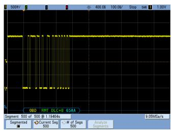
The oscilloscope should have just captured and decoded 500 consecutive CAN frames. Let's now review all of the CAN frames and determine how long of a time-span the oscilloscope just captured.
