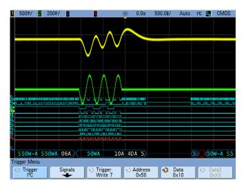
The oscilloscope should now be triggering on a Write operation to Address 50 hex with an Acknowledge (50WA), followed by a data byte value of 10 hex with an acknowledge (10A). This particular trigger condition is coincident with a transmission of a 3-cycle analog chirp shown on channel 1 (yellow waveform) and channel 2 (green waveform). Let's now view the I<sup>2</sup>C decoded data in the "lister" format.
