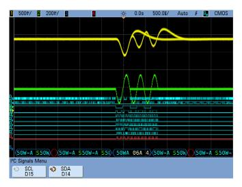
You should now be able to view the time-aligned serial decode trace at the bottom of the display showing  $I^2C$  decoding of D14 (SDA). But the oscilloscope is not yet triggering on  $I^2C$ . It is still triggering on an edge crossing of channel 2. Let's now set up the oscilloscope to trigger on a Write operation to address 0x50hex with an Acknowledge, followed by a data value of 0x10hex.
