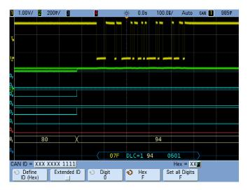
The oscilloscope should now be triggering on frame 07F. Because "F" is unique in the lower nibble of the ID for our demo board signal, specifying the upper two nibbles (07) is not necessary in order to trigger on 07F hex. Let's now make some time-correlated measurements across analog, digital, and serial bus signals.
