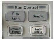
Because the oscilloscope may have been used in a variety of applications by a variety of people, it is a good measurement procedure to put the oscilloscope in a known starting mode (Default Setup). This will make it easy to duplicate measurements because no special conditions will be set.
