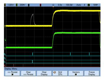
With the infinite persistence mode, all repetitive and "historical" acquisitions are accumulated and displayed on screen. This can be very useful when setting up an overnight measurement to capture an elusive event. Let's now set up a glitch trigger condition that will trigger exclusively on the anomaly.
