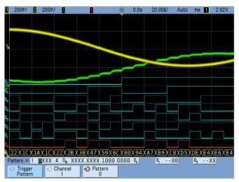
The oscilloscope should now be triggering on pattern "80h" of B1 while channel 1 is low (or below its trigger level).
