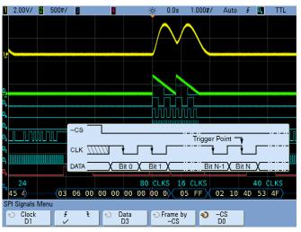
Let's now set up the oscilloscope to trigger on a specific SPI transmission of data (02 10) in order to synchronize acquisitions coincident with a specific burst of the analog signals.
