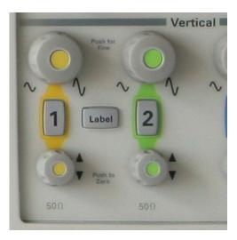
channel 1 menu. Press again to turn the channel on and off.
