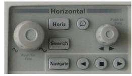
Observe the changes in the displayed signal. The current time base setting is displayed at the top of the display on the status line.
